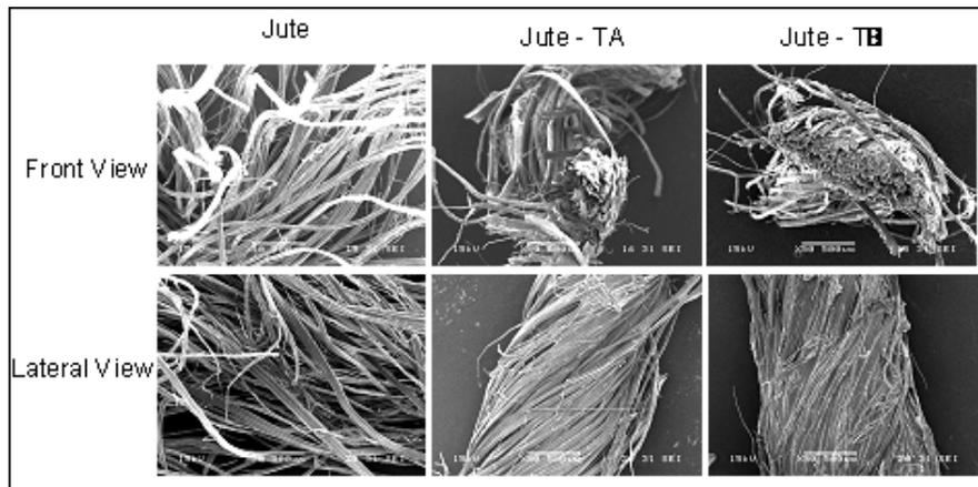
Fig. 2 SEM images of jute fibers with and without PHB treatment.
