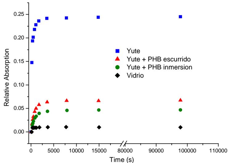
Fig. 1 Humidity absorption test results.
